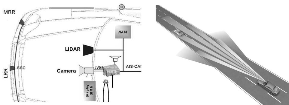
**Figure 1:** Sensors connected to an ECU. The sensors deliver data e.g. for obstacle detection
