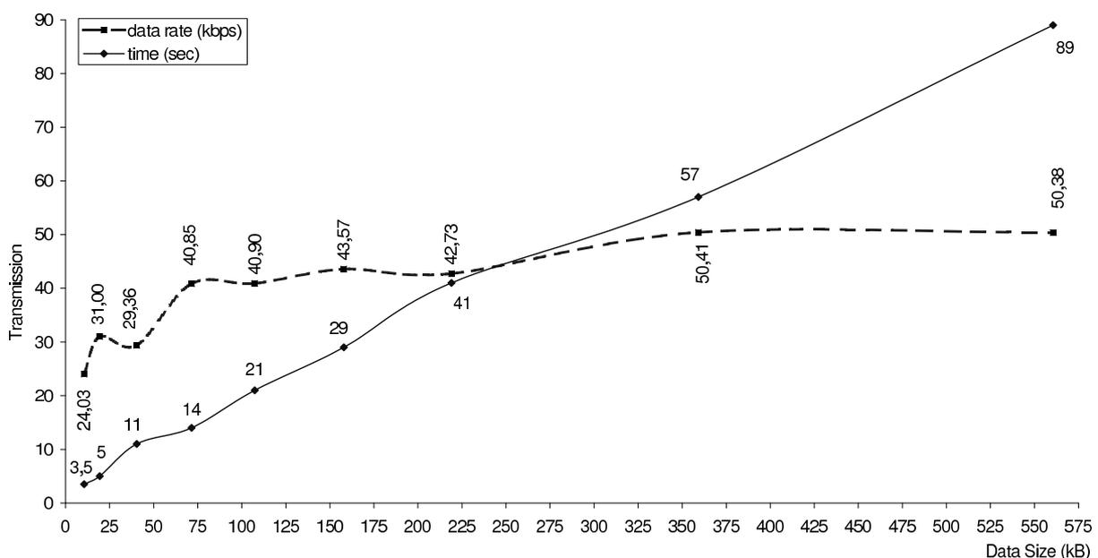
Figure 6: File Upload Transfer Rates using Class 10/12 GPRS Modems
